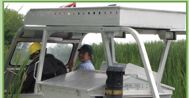
Riding shotgun on the USFWS amphibious Marsh Master mower during Phase II summer (2015) mowing (one component of Brockport cattail control methodology).
